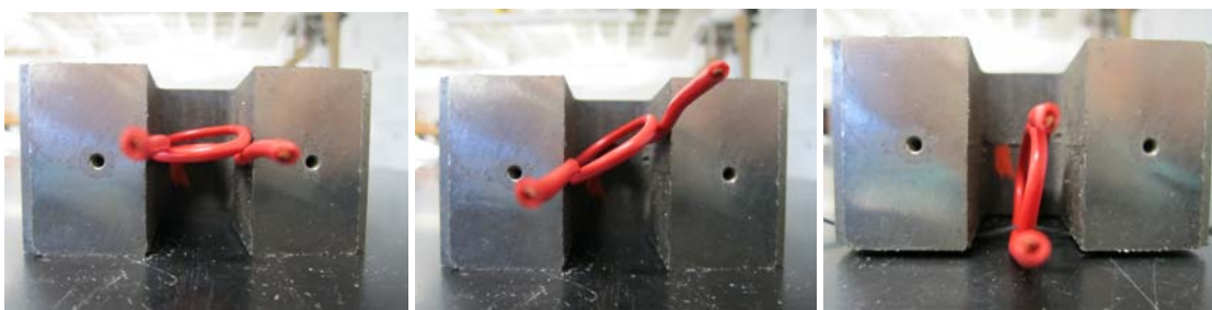
Figure 3: Schematic diagram showing the difficulty with a coil in a magnetic field.
